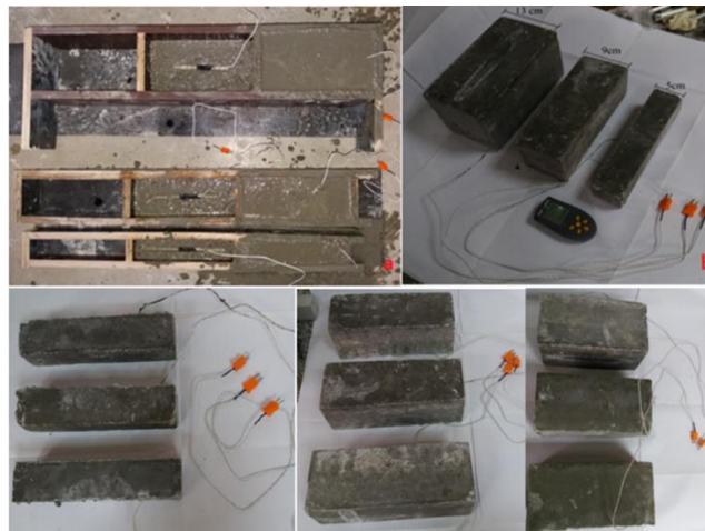
Figure 1. a) Thermocouple attached to GFRP bar b) samples with different concrete covers (20-40-60 mm).
