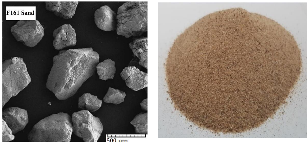
Figure 1. Firoozkuh sand (F161) used in this study and scanning electron microscopic (SEM) image of this sand.
