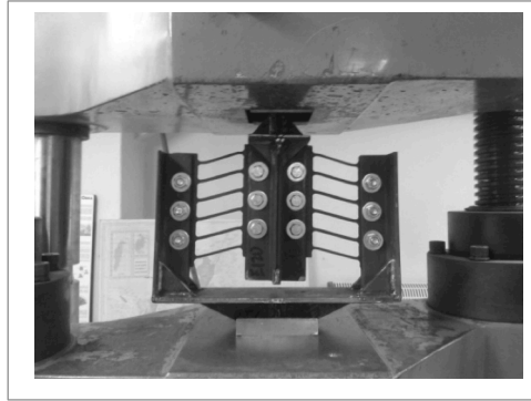
Figura 5. Montaje del ensayo de caracterización mecánica del disipador con placas ranuradas Figure 5. Assembly of the mechanical characterization test of the dissipation device with slit plates
