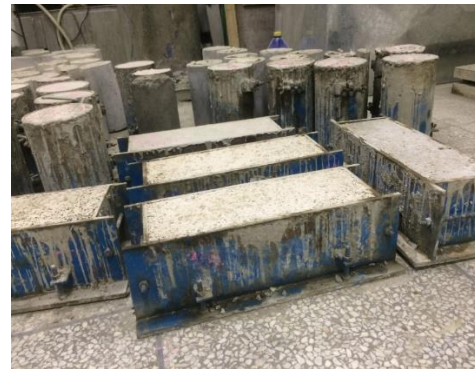
Figure 3b. Beams and cylinders after casting
