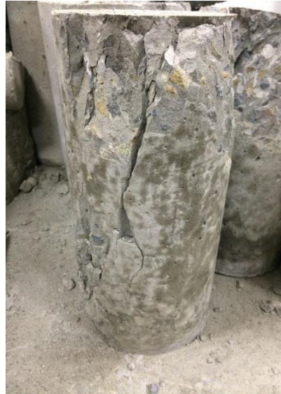
Figure 12b. Cylinder after compression test
