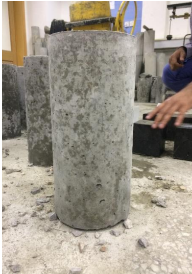
Figure 12a. cylinder before compression test
