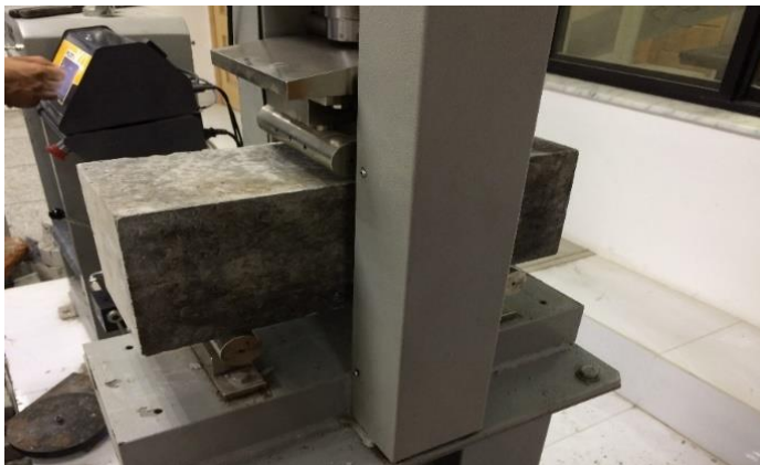
Figure 8. Flexural testing of beam specimen
