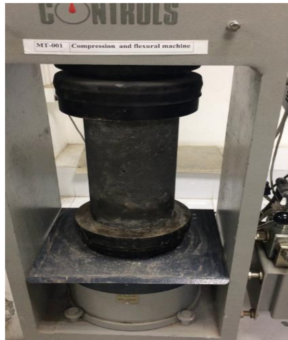
Figure 6. Compression testing of cylinder
