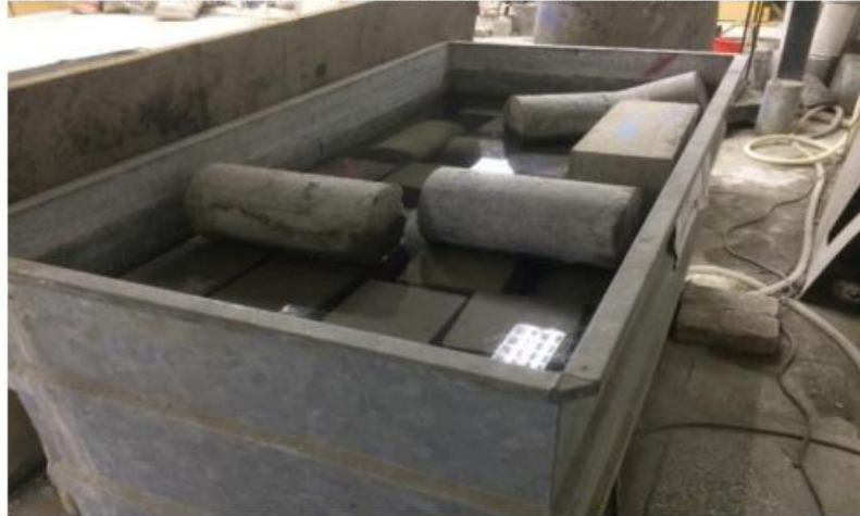
Figure 4. Specimen in curing tank
